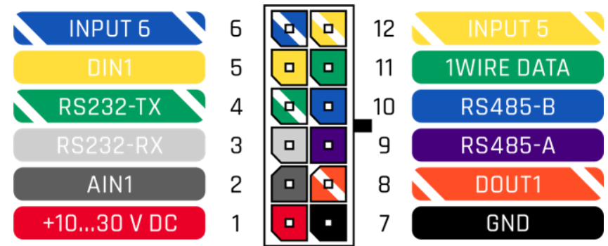
Figure 2 FMU125 2x6 socket pinout
